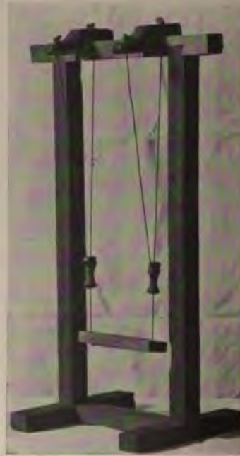
FIG. 203.—Model of child's swing. Movable hollow hand-pieces slide upon the perpendicular ropes. Cords passing from these hand-pieces to wooden arms permit child to swing herself. Excellent for out-door exercise.
